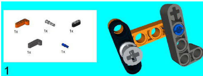
Figure 6-35. Start with two 4 x 2 Angular Beams and a 3M Beam. Use a Snap with Friction and a Connector Peg/Cross Axle to join them together.
