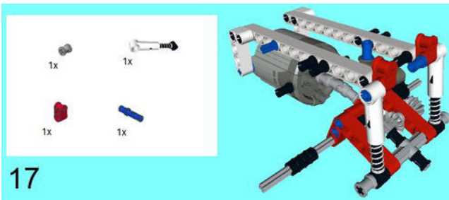
Figure 5-18. A Shock Absorber joins with a 3M Connector Peg, a Technic Cross Block (1 x 2), and another Technic Cross Block (1 x 3). This time, it is on the other side and secured with a Bush.
