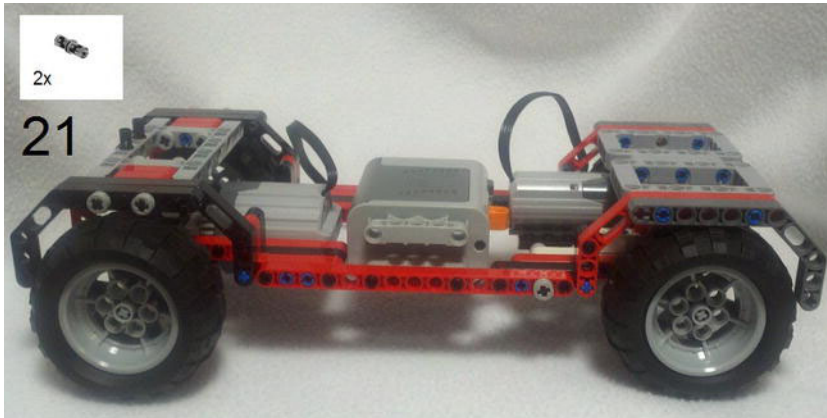
Figure 3-29. When both motors are connected to the IR-RX, you can access them with an IR controller—provided the battery box is turned on and everything is properly connected.
