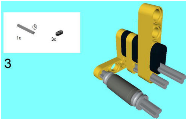
Figure 6-21. Attach three 2M Levers to another 5M Axle and then join the 5M Beam.
