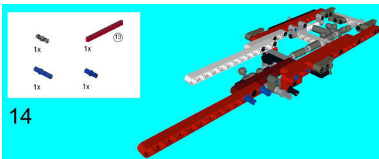
Figure 7-54. Add another long 13M Beam here via a Connector Peg, 3M Connector Peg, and a Connector Peg with Cross Axle.
