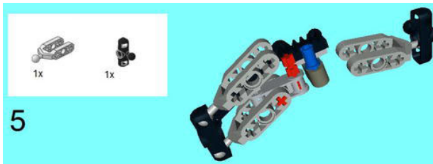
Figure 5-28. Another Steering Knuckle Arm joins with a Steering Arm in a ball-and-socket, almost a mirror image of the other side.
