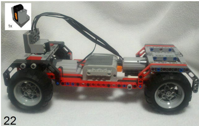
Figure 3-30. An IR-RX IR receiver is connected to the M-Motor for steering to the blue Power Functions Port and the XL-Motor for propulsion is connected to the red Power Functions Port. This model, with the IR-TX remote control, is ready to go.
