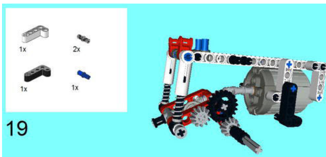
Figure 5-20. A Connector Peg/Cross Axle joins two 4 x 2 Angular Beams together, and joins the 13M Beam and XL-Motor. Don't forget the two Connector Pegs at the bottom of the 4 x 2 Angular Beam as shown.
