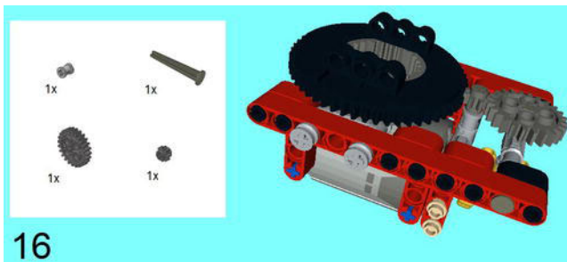
Figure 6-17. Another 4M with Stop and Bush join with the 180 Degree Angle Element in front of the construction. Now that this is secured in place, put the Gears on it as shown, and be sure they mesh together.
