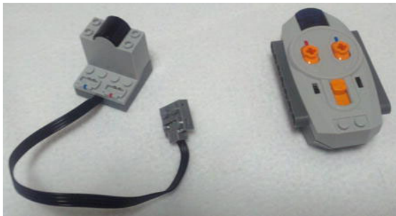
Figure 3-4. On the left is the IR-RX with its red and blue power sockets. On the right is the IR-TX with its red and blue controls.
