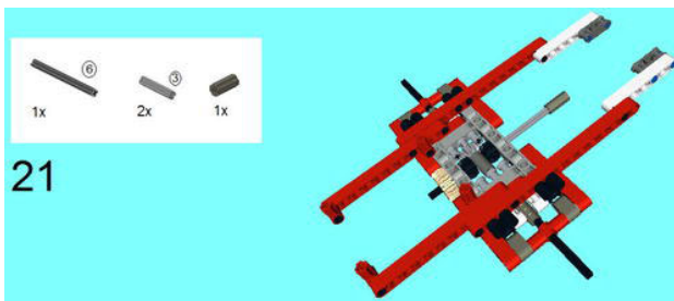
Figure 5-71. Two 3M Axles join here on the 180 Degree Element, along with a 6M Axle. Note the Cross Axle extension on the middle.
