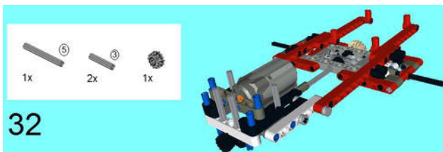
Figure 5-82. Note the placement of the Z12 Gear Wheel on the bottom, as well as the new 5M Axle. The 3M Axles go on each side, inserted into the 4 x 2 Angle Beams.
