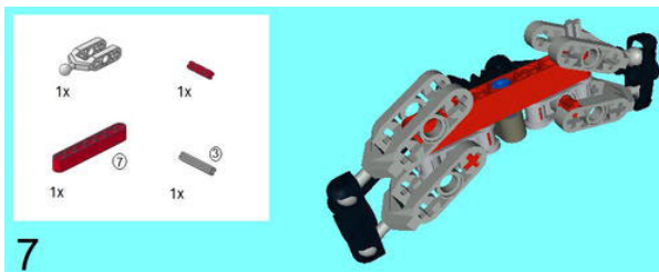
Figure 5-30. Insert a 2M Axle to join the Steering Knuckle Arm with the Double Cross Block. Another Steering Knuckle Arm joins here, and a 7M Beam joins the two sides together. Don't forget to add the 3M Axle vertically on the Double Cross Block.
