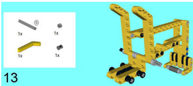
Figure 6-31. Add a 5M Axle with a Bush. Insert a 3 x 7 Technic Beam with the Half-Bush.
