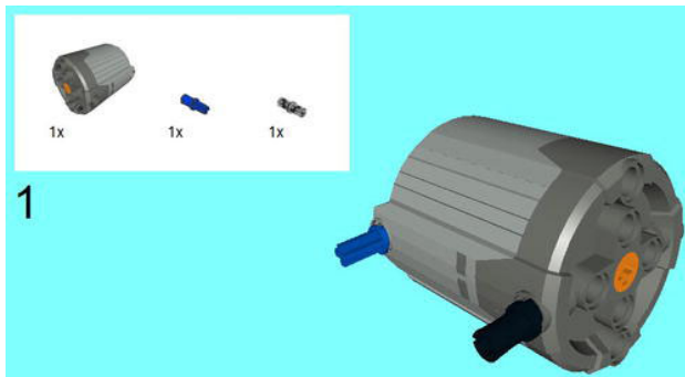
Figure 5-2. Start with the XL-Motor and insert a Connector Peg and Connector Peg/Cross Axle as shown.
