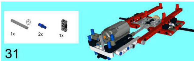
Figure 5-81. Place a Double Cross Block on the bottom with a 5M Axle extending from it, along with two Connector Peg/Cross Axles.
