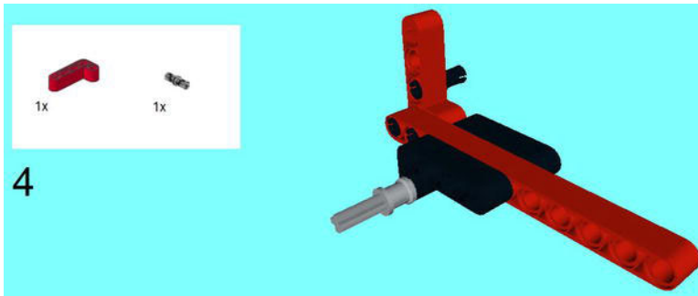
Figure 2-30. A 4 x 2 Beam fits on the end with two Connector Pegs and one in the middle.
