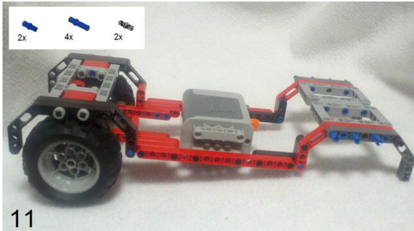
Figure 3-41. Attach the double-engine section from Project 3-2 to the basic LEGO frame from Project 2-1.
