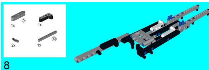
Figure 7-74. Attach a 13M Beam with a 4 x 2 Angular Beam with Connector Pegs. Don't forget to add the 5M Beam.
