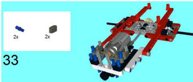
Figure 5-83. Two of the Cross and Hole pieces go on the 3M Axles, and two Connector Pin/Cross Axles go in on the 4 x 2 Angle Beams.
