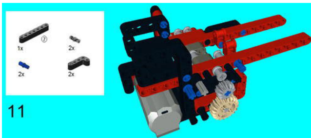
Figure 6-70. Another 7M Beam joins the construction on this other side, and lines up here with two 4 x 2 Angular Beams. Note the placement of the Connector Peg/Cross Axles and Connector Pegs.
