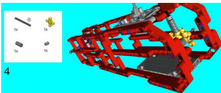
Figure 7-97. A 6M Axle with Angular Gear, Tube, and Bush join here to mesh with the Angular Gear as shown.
