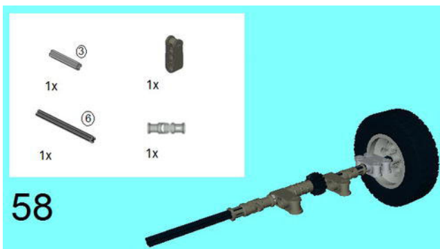
Figure 5-108. Again, add some essential parts to the axle: a 3M Axle, a 3M Cross Block, a Universal Joint, and a 6M Axle, in that order.
