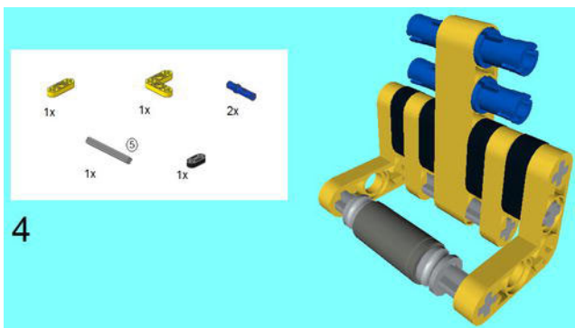
Figure 6-22. To complete the end of the scoop, add another 5M Axle to an additional 2M Lever, 3M Lever, and 3 x 3 90 Degree Lever. Add two 3M Connector Pegs to the 5M Beam.
