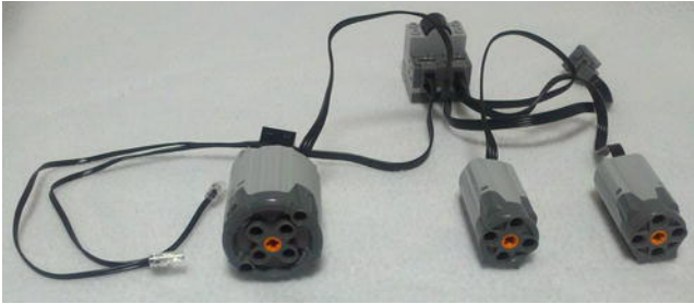
Figure 3-5. The IR-RX is capable of working four Action elements at once, provided two are being worked at the same time.
