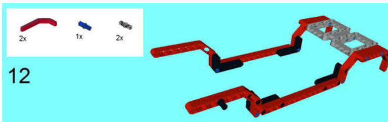
Figure 2-23. A Double Angular Beam is added to the construction to form a fender shape. This only uses one Connector Peg, and another Connector Peg and Connector Peg with Cross Axle join the 5 x 3 Angular Beam.
