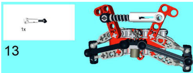
Figure 5-36. The Shock Absorber piece joins with the Connector Pegs on the Angular Beams here. This will keep the Track Rods at different angles.
