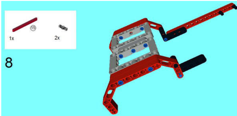
Figure 2-19. Connect a 15M Beam to the end of the 5 x 3 Angular Beam, and insert two Connector Pegs to that Beam as shown.
