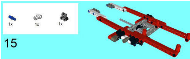
Figure 5-65. This step is similar to Steps 3 and 13, with a Technic Cross Block, a Zero Degree Element, and Connector Peg/Cross Axle.
