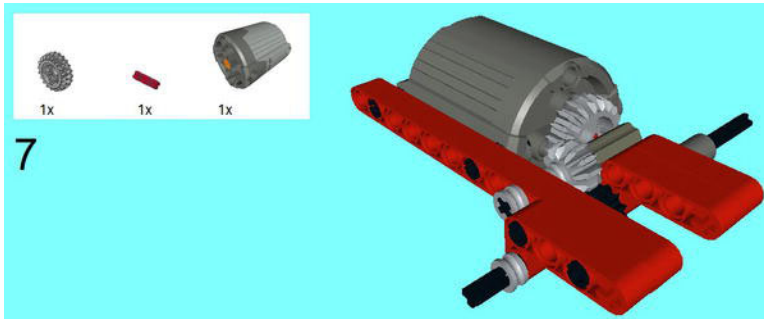
Figure 2-48. The XL-Motor needs a 2M Axle, as well as a Double Conical Wheel Z20. Before the M-Motor is connected to the pegs from the last step, it must mesh perfectly with the gear. These things need to fit together tight, but not too tight.
