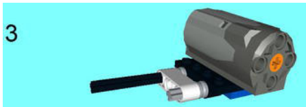
Figure 3-11. Instead of leaving a studded section, it is actually half of one. At this point, the pieces assembled in step 1 and step 2 now join up as shown, with 1M of both axles joining with the Technic Bearing Plate of the left side of the M-Motor.
