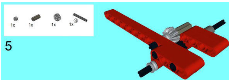
Figure 2-46. In this step, a 4M Axle is connected to a Cross Axle Extension. Then another Conical Wheel (12 Teeth) is added, and this must mesh perfectly with the other gear. A Half Bush is attached there and then inserted in the hole as shown.
