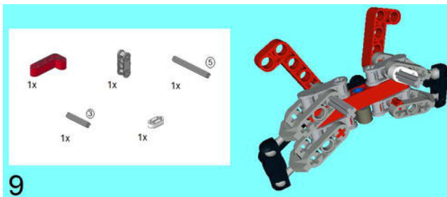
Figure 5-32. Add another Double Cross Block, 5M Axle, and 4 x 2 Angular Beam. Add another 3M Axle vertically through the two Double Cross Blocks on the left and a 2M Lever on one of the 5M Axles.
