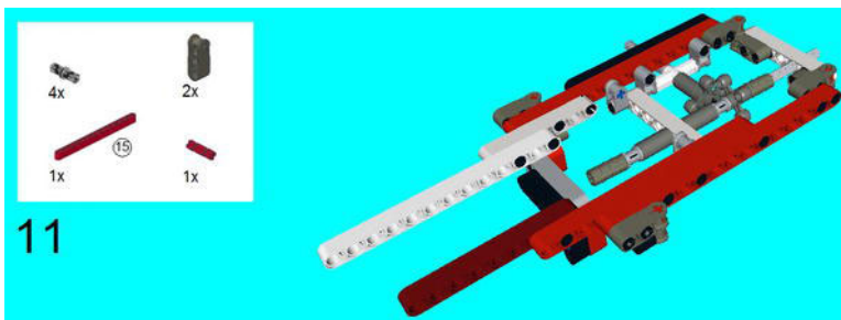
Figure 7-51. Add a 15M Beam on one side with a 3M Cross Block on a 2M Axle.
