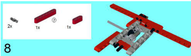
Figure 5-58. A Connector Pin joins a 7M Beam with the H-Frame, and a 3M Beam joins the H-Frame.
