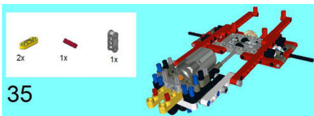
Figure 5-85. The 3M Levers go atop the other levers, the 2M Axle goes between them, and a Double Cross Block goes atop that.
