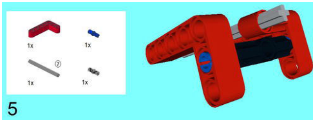
Figure 5-6. Insert the 180 Degree Element on the connector pegs, with a 5 x 3 Angular Beam. Place a 7M Axle in the Zero Degree Element so it is 1M on one side and 5M on the other.
