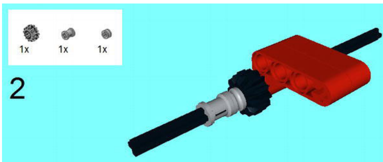
Figure 2-43. A Double Conical Wheel (12 Teeth) is placed on the left side of the axle, with a Bush and a Half Bush.
