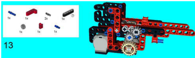
Figure 6-72. Attach the 5M Beam to the construction and attach a Z12 Gear so it meshes with the other one as shown. Attach the Cross Block and the 4 x 2 Angular Beam as well.
