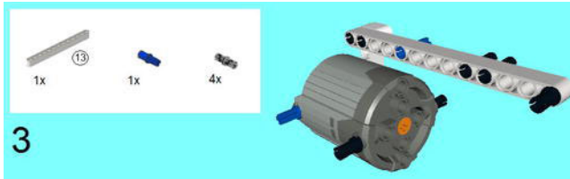
Figure 5-4. Add a 13M Beam to the 4 x 2 Angular Beam, along with the Connector Pegs and Connector Peg/Cross Axles. Add another Connector Peg to the XL-Motor.
