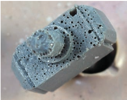
Figure 4: Foaming on a resin part.
